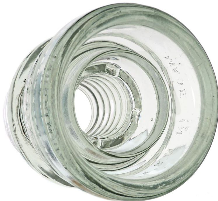
DETAIL OF THE FOUR NOTCHES AROUND THE BASE OF THE THREADS
