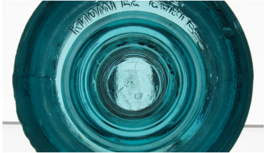
NOTE THE CONCENTRIC CIRCLES IN THE TOP OF THE PINHOLE (NOT AN ELMER RING). THIS WOULD ALSO SEEM TO INDICATE A FRESHLY MADE PLUNGER.
